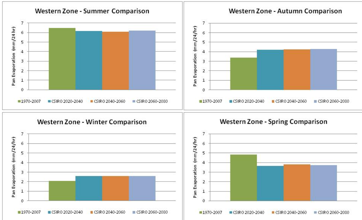
Figure 44 - Seasonal comparison of pan evaporation for historic interdecadal time periods and future time horizons
