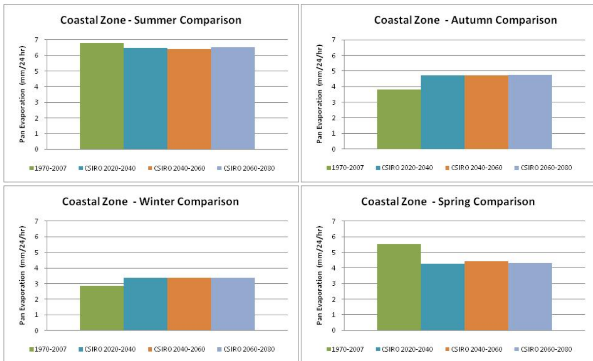
Figure 43 - Seasonal comparison of pan evaporation for historic interdecadal time periods and future time horizons
