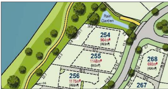
Figure 9: Design plans with the inclusion of Water Smart Measures (see rain garden label). (Source: Stocklands)
